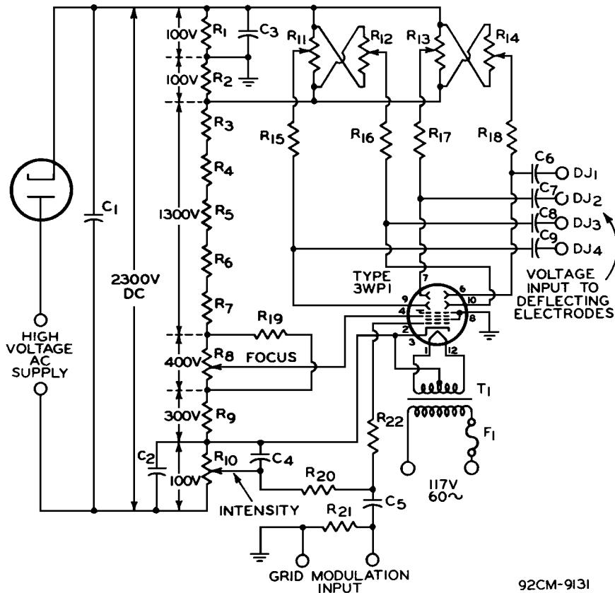
C1: 0.5  $\mu$ f, 3000 voltsC2: 8  $\mu$ f, 250 voltsC3: 1  $\mu$ f, 200 voltsC4: 1  $\mu$ f, 200 voltsC5: 0.05  $\mu$ f, 3000 voltsC6 C7 C8 C9: 0.05  $\mu$ f, 600 volts
