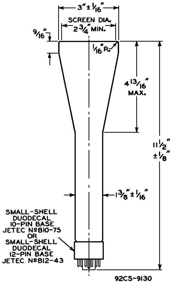
LINE OF BULB WILL NOT DEVIATE MORE THAN  $2^\circ$  IN ANY DIRECTION FROM PERPENDICULAR ERECTED AT CENTER OF BOTTOM OF BASE.
